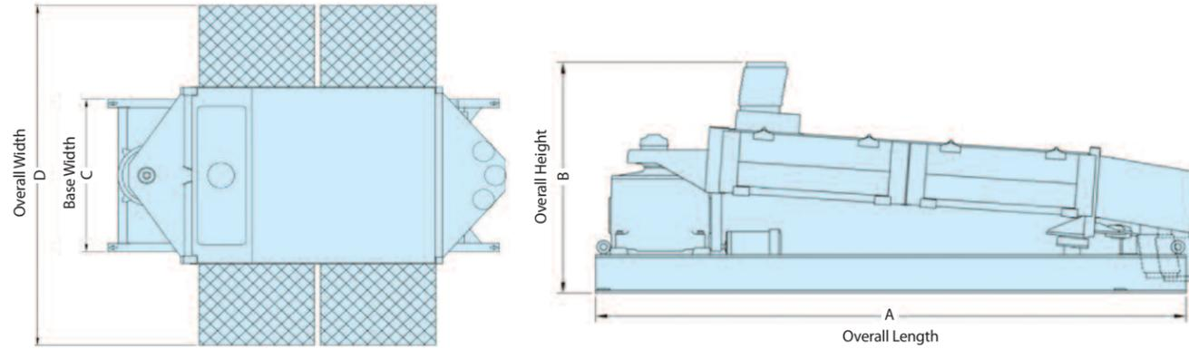
The following specifications are for Apex Screeners of standard construction, ranging from a single surface models (two grades – one separation) to a three surface models (four grades – three separations). Drawings are representative, but overall dimensions may vary depending on the mounting method.
